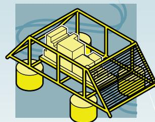
Offshore **seafloor robots** operate, modify, and install small parts in dangerous areas previously serviced by human divers
